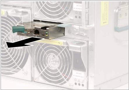
Figure 64: Removing the management blade
